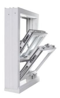
To close the window, simply push the sash back towards the outer frame and the top sash. You will hear a 'click' as the spring loaded snap latches lock back into the outer frame. Once the tilt restrictors have been re-engaged, the window can be moved up or down as required.
