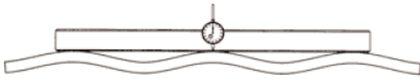
Figure B.3 — Set the zero of the gauge on a peak of the roller wave
