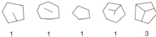
Figure 21 — Examples of crack-free particles and the assessment regarding the number
